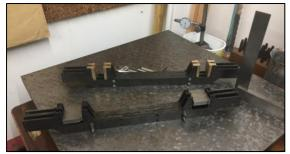
machine the horn guides to size. Very much like one would do so with the frames of a steam loco. Luckily, I have most of a box of slip gauges that I rescued from the stores scrap bin of a company I worked for. They were no longer suitable for the precision work they
