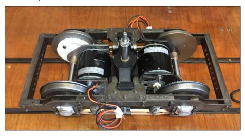
Later on in the final assembly I did have to come up with an alternative solution to that shown on the Dan Jeavons drawings of holding the motors in place to stop them rotating around the axle as all 4 motors hang on the axles and have to mesh with a gear attached to the relevant wheel.
