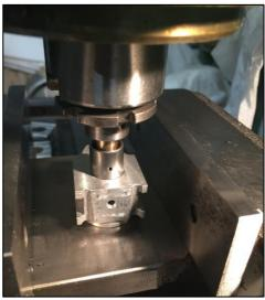
another company, after buying the castings from Dan Jeavons, with much more substantial ones which I had recently purchased which would not deform with the torque of the motors. The new motor mounting plates had the oilite bushes Loctited in place.
