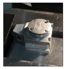
total of 32 x 12BA holes into the axle box castings to retain them. I also deviated away from the drawing by replacing the oilite bearings called for on the drawing with needle roller bearings. The bearings had a small hole in the outer cage so I drilled a hole through from the top of the axle box to line up with this before pressing in the bearings so that I could put a drop of oil down this for lubrication when required.
