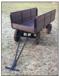
The wooden sides have been replaced with plastic planks held in place with stainless steel fastenings.
